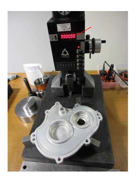
Measure dimension S2 on secondary line (cover side)
