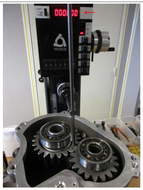
Measure gap G between primary and secondary lines on secondary 6th gear.
