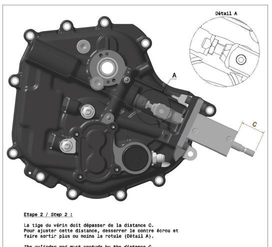
The cylinder rod must protude by the distance C. To adjust this distance, loosen the lock nut and adjust the ball joint (Detail A).
